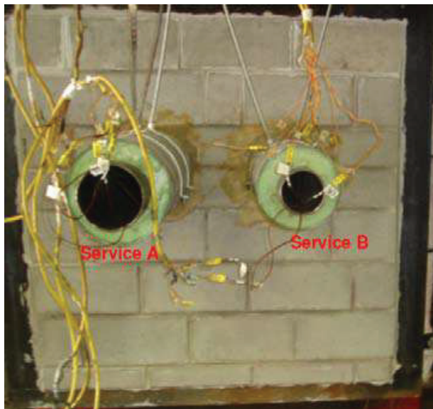
Unexposed face of test specimen prior to commencement of test
