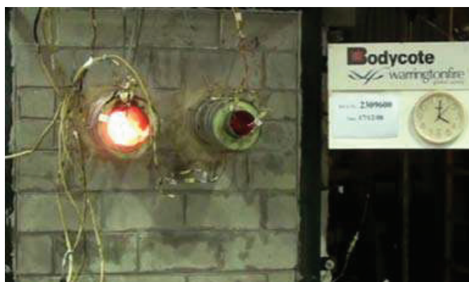
Unexposed face of test specimen after completion of test duration 240 Minutes
