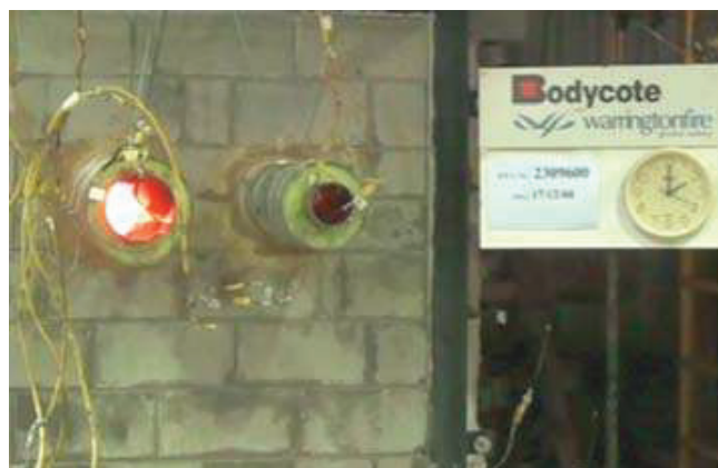
Unexposed face of test specimen after approximately 120 Minutes test duration
